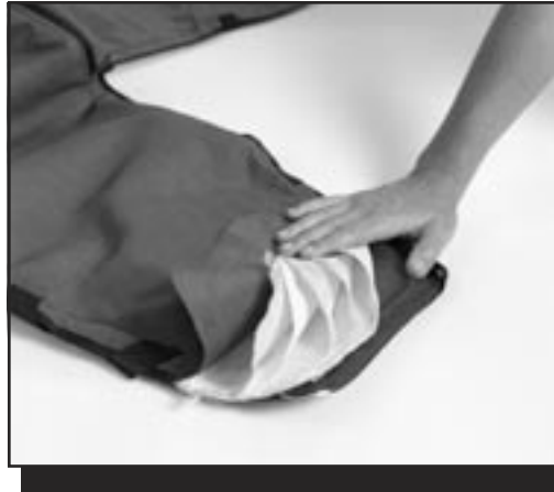
Figure 1—A chain saw chap has five layers of Kevlar that jam the chain saw's drive sprocket, stopping the chain saw and preventing injuries.
